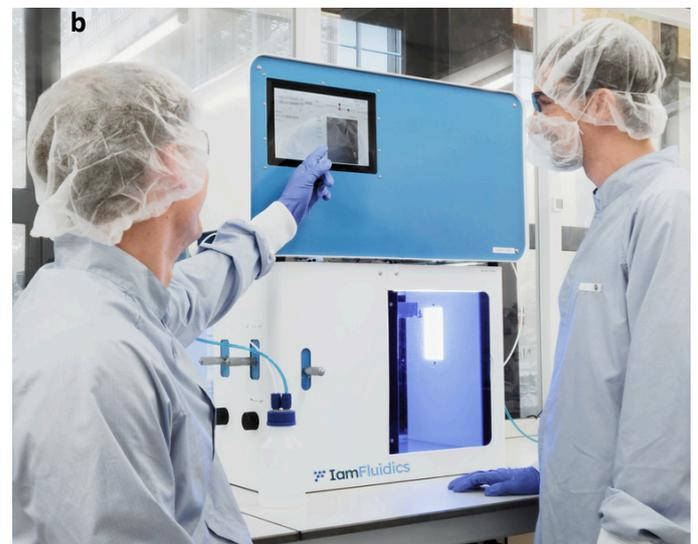
**(b)** Lab-scale IN-AIR-MICROFLUIDICS™ machine for cleanroom-grade production up to kilograms per day.
