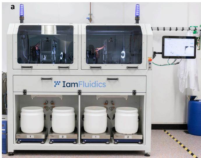
**(a)** Industrial-scale IN-AIR-MICROFLUIDICS™ machine to produce multiple tons of microparticles per year.
